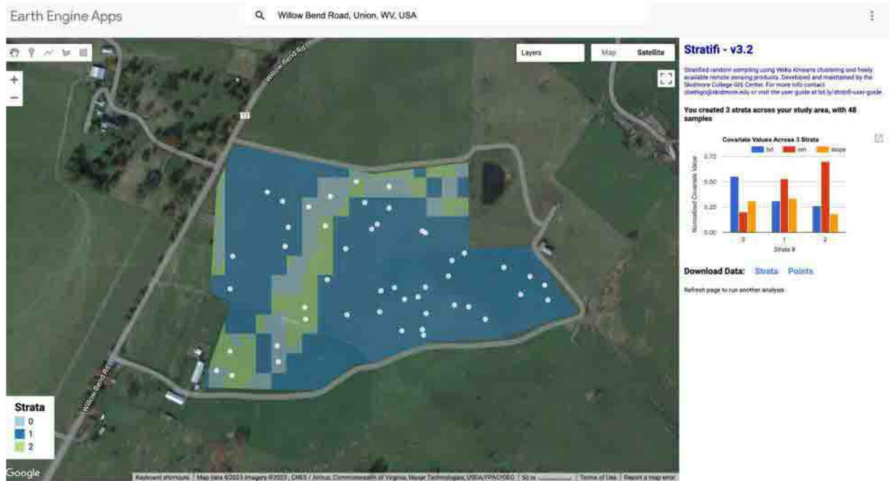
Figure 2. Output from the Stratifi app of an example farm (WVU-owned) using slope, POLARIS organic matter, and bulk density estimates as stratification parameters. Using our knowledge of this farm's landscape and history as well as Stratifi, we would only sample from Strata #1 (dark blue) at the randomized points indicated. The GPS coordinates for the points can be downloaded and used in-field.
