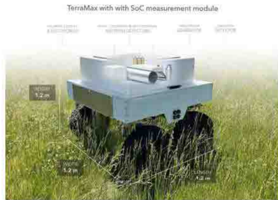
Figure 4: TerraMax RECAR (Robot-Enabled Carbon Radiological) Measurement System
