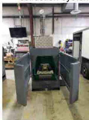
Figure 2. GreenFeed GHG data collection system
